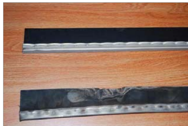
New bat (top) and worn bat (bottom).
